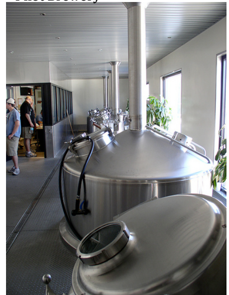
Main floor of the pilot brewery. Kettles front to back - Mash Tun, Lauter tun, Boil 1, Boil 2, Whirlpool.
